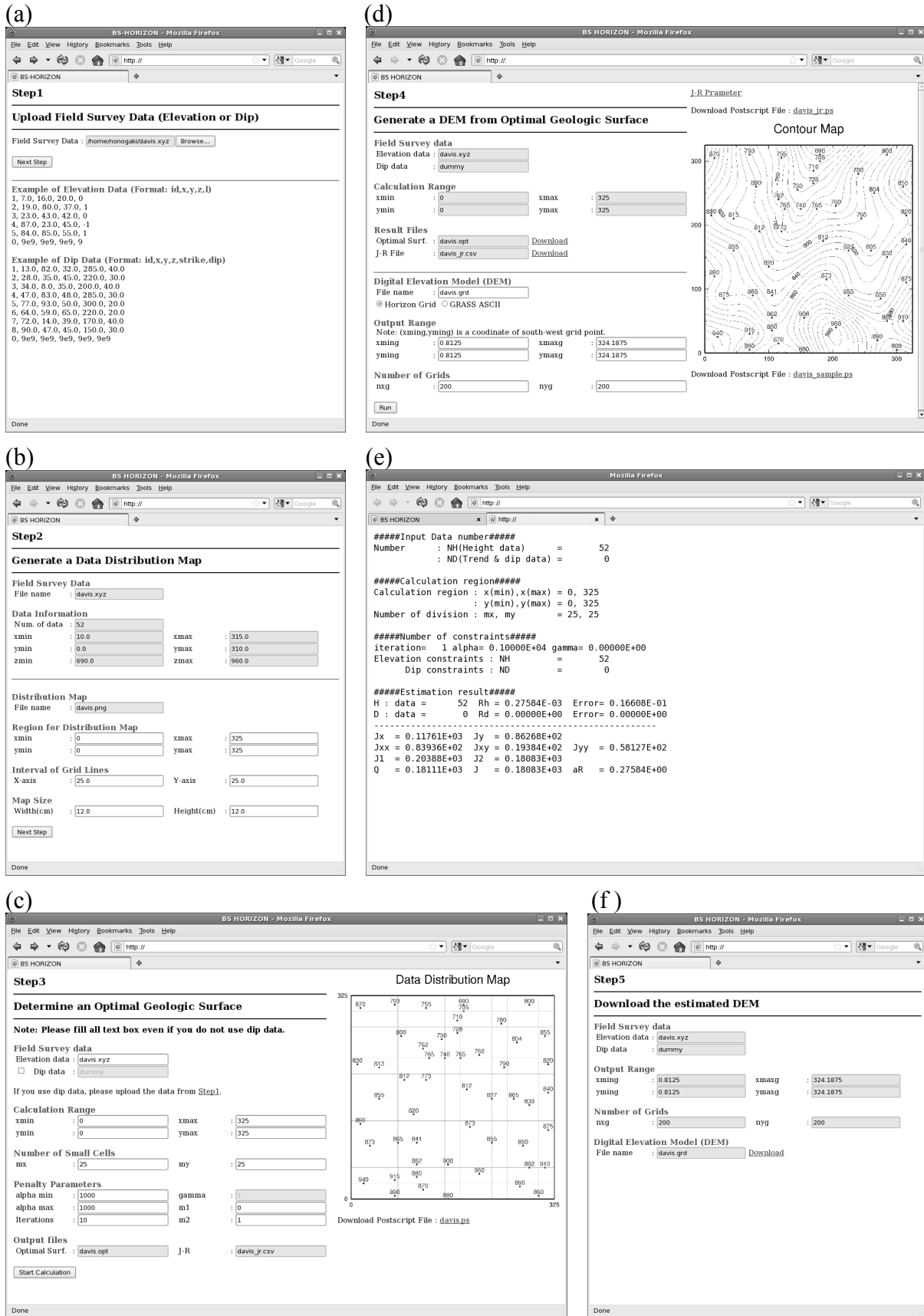
Figure 2. Example of operation screens. (a) data upload screen, (b) distribution map generation screen, (c) optimal determination screen, (d) DEM generation screen, (e) functional evaluation screen and (f) data output screen.
